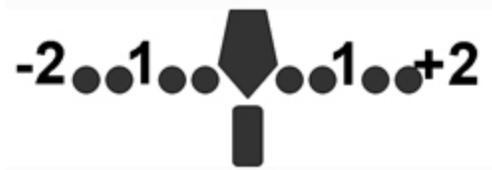
A light meter is an instrument inside your camera that tells you if the amount of light reaching the film will be enough or too much to properly expose your image. The light meter takes into account your shutter speed, film speed, and aperture settings.
