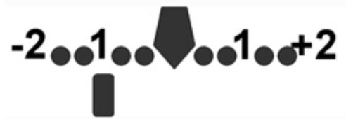
Your camera's light meter shows you the amount of light in aperture settings. Each dot on the meter represents a partial "stop", or aperture increment. The numbers represent whole stops. Even though your F-Stop setting controls the aperture itself, the meter readings will also change if you change your film speed or shutter speed.
